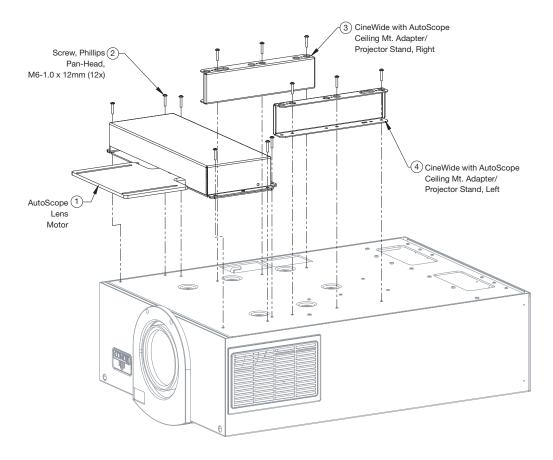
✓ Installing the AutoScope Lens Motor (VX-33d/CineWide with AutoScope)
